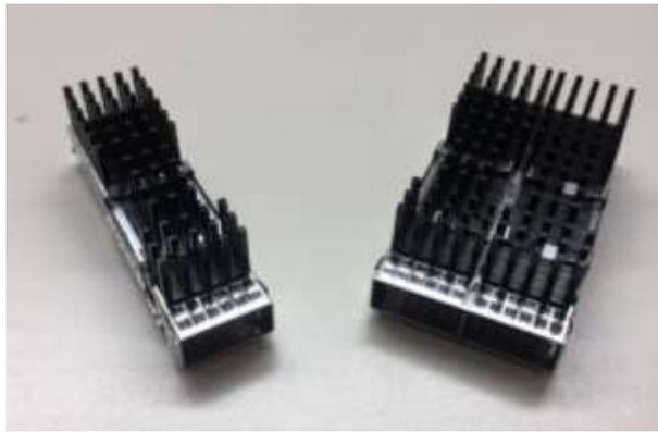
Figure 7: QSFP-DD single card cage
