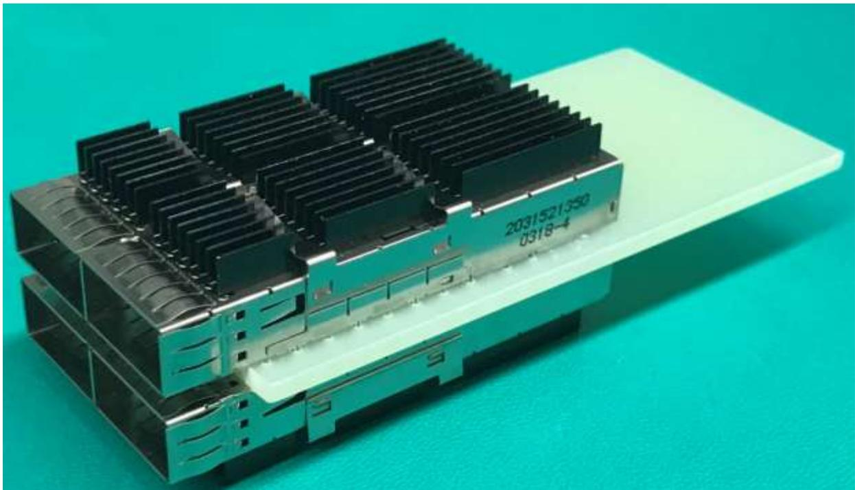
*Figure 9: Belly to Belly QSFP-DD card cages*
