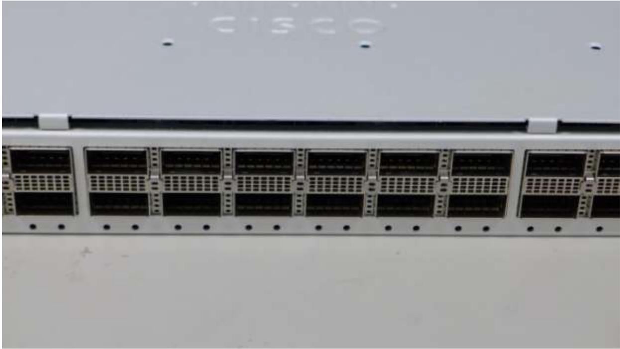
*Figure 10: Stacked QSFP-DD cages*
