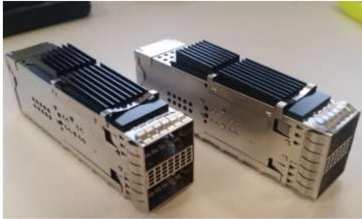
Figure 6: QSFP-DD Stacked card cage
