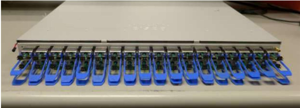
Figure 20: 1U switch with 36 stacked QSFP-DD cages used to generate thermal test data in Figure 19
