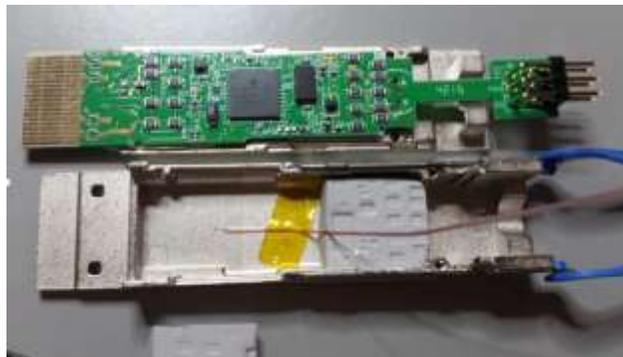
Figure 17: Thermal Couple inside module case near center of HS pedestal
